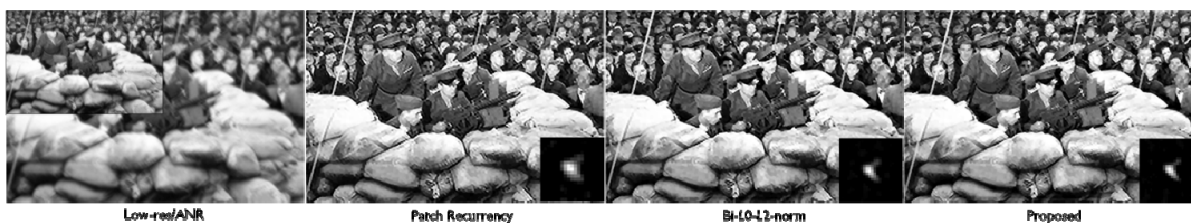
Figure 6. Blind super-resolution (2 times) by ANR [11], Patch Recurrency [16], bi- L_0 - L_2 -norm [18], and the proposed approach.
