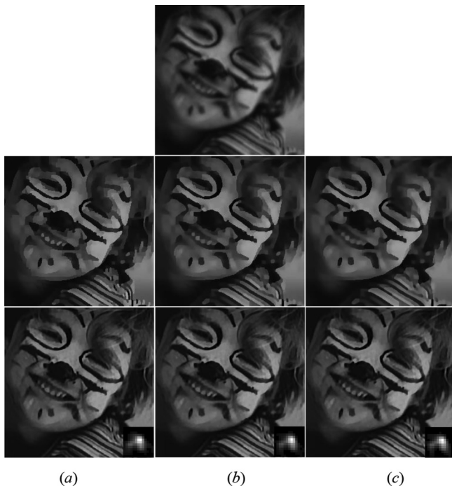
Fig. 2. Sensitivity analysis of the proposed model (1) on the spatial scale \sigma . The first row presents the blurred image image04-kernel05 ( 225 \times 225 ) from the dataset of Levin et al. [19]. The intermediate image and final deblurred image accompanied with the estimated kernel corresponding to each setting of \sigma are provided in each of three columns (from the second to the third rows). The PSNR of final deblurred images are: (a) 34.92 dB ( \sigma = 1 ); (b) 34.66 dB ( \sigma = 3 ); (c) 34.11 dB ( \sigma = 5 ).
