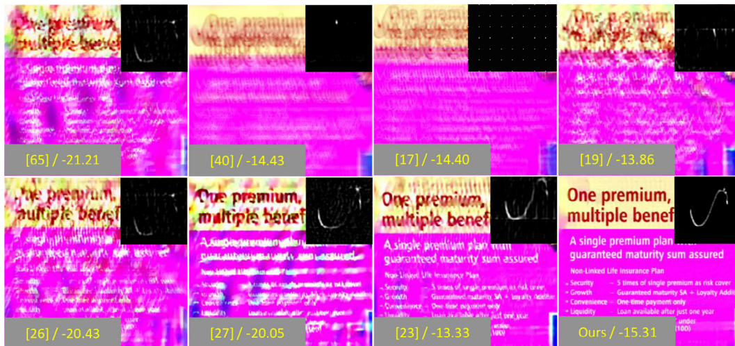
Fig. 9. Deblurring results of the blurred image text04-kernel04 in the dataset Lai et al. [2] corresponding to the top eight approaches in terms of PSNR/SSIM. The value of no-reference metric [67] is shown in each image for visual perception assessment. Their PSNR/SSIM values are [65] (13.63 dB/0.5611), [40] (13.72 dB/0.5634), [17] (13.74 dB/0.5605), [19] (13.83 dB/0.5903), [26] (13.91 dB/0.5724), [27] (14.03 dB/0.6386), [23] (16.30 dB/0.7166), Ours (21.43 dB/0.8437).
