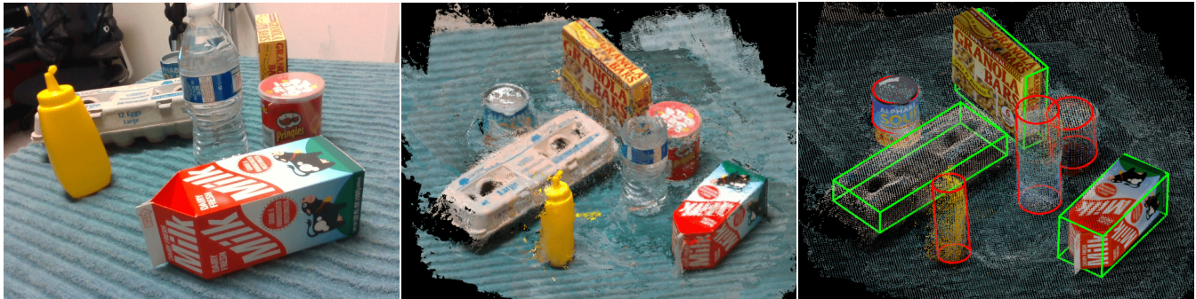
Fig. 1. LEFT: Input to the system is a sequence of RGB images from a camera-in-hand. MIDDLE: Reconstructed point cloud. RIGHT: Multi-level scene representation, including 3D point cloud (downsampled for better visualization), primitive shapes (cylinders and cuboids), and known object CAD models (granola bars, milk, and soup can).
